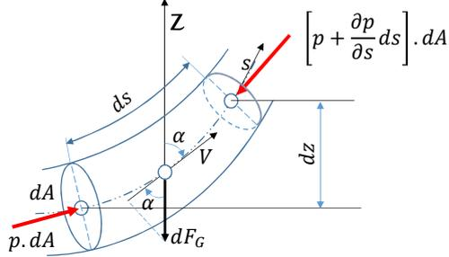
$$\frac{\partial V}{\partial t} + V \frac{\partial V}{\partial s} + \frac{1}{\rho} \frac{\partial p}{\partial s} + g \frac{\partial z}{\partial s} = 0$$
